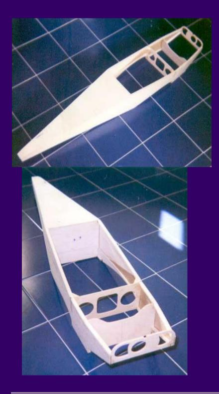
• 15 May 2002 - ailerons shaped and hinges installed. Fuselage sides cut out and longerons fitted.
