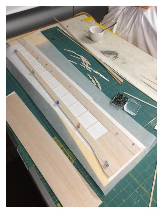
12. Glue the front and rear dihedral braces to the spar, then thread the ribs onto the spar and glue this assembly into position over the sheeting and cap-strips. PVA works well here. Glue the false LE in place.
