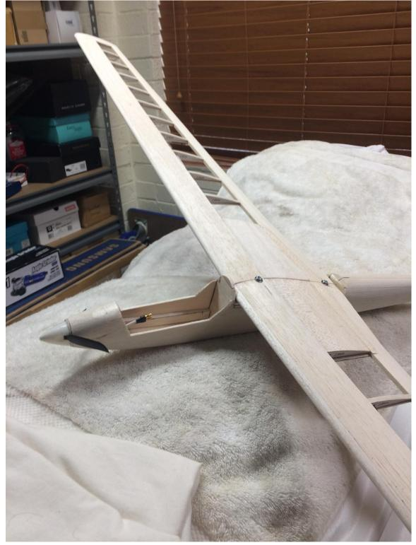
18. Make up the fuselage over-wing fairing as shown on the plans, and temporarily fit in place to shape. The model is now structurally complete, and should look something like this:
