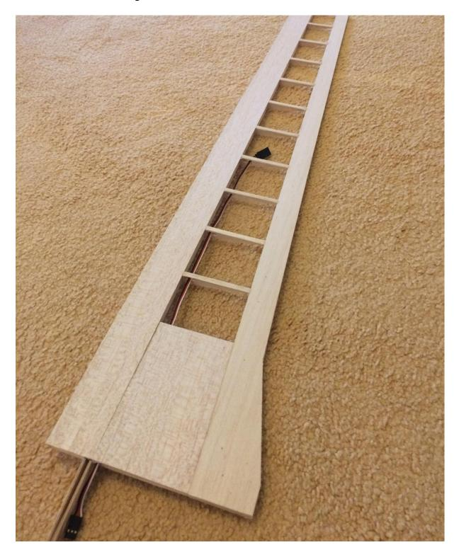
16. Build the right wing over the plan, propping up and joining the left wing to the right wing during construction before the top sheeting is added. A hole is made in the bottom RHS centre-section sheeting for the aileron servo leads to exit.
