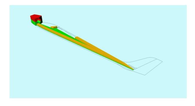
4. Chamfer the rear of the fuselage doublers where the sides will be drawn together
