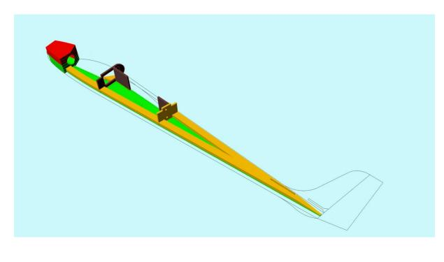
6. Glue fuselage LHS assembly to fuselage RHS assembly.
