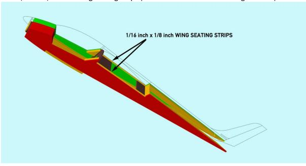
Glue the 6.4mm balsa forward fuselage bottom sheeting in place, as well as scrap 1/16" x 1/8" balsa wing seating strips (which are to allow for the wing dihedral).
