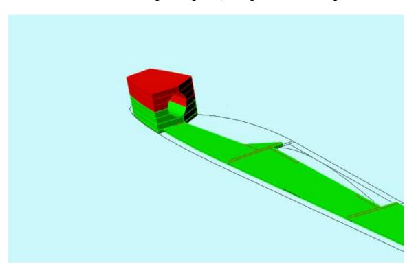
3. Glue the 6.4mm balsa fuselage doublers to the fuselage RHS as shown. Separately, glue the 6.4mm balsa fuselage doublers to the fuselage LHS.
