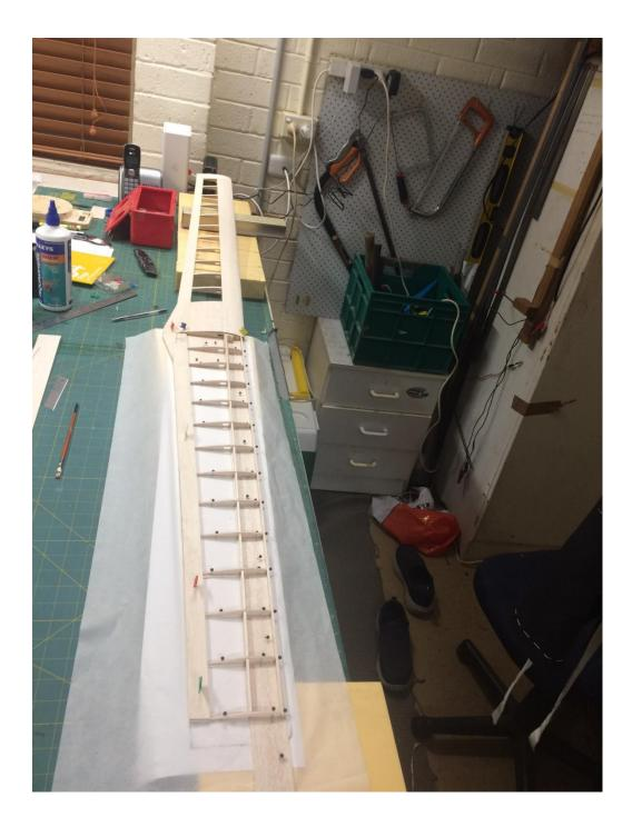
17. Once the wing structure has been completed, drill holes for 2 x 4mm wing bolts (use location shown on the plans) then present wing up to fuselage, marking the position on the ply fuselage wing mount plates where the bolts come through. Drill and tap holes for the 4mm bolts in the ply or for alternative blind retention nuts.
