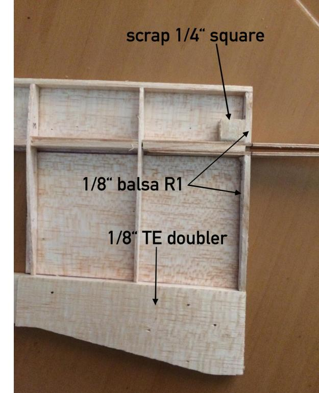
13. Fit and glue front and rear sections of 1/8" (3.2mm) balsa root rib R1, as well as TE doubler and scrap ¼" square balsa front wing bolt reinforcement.
