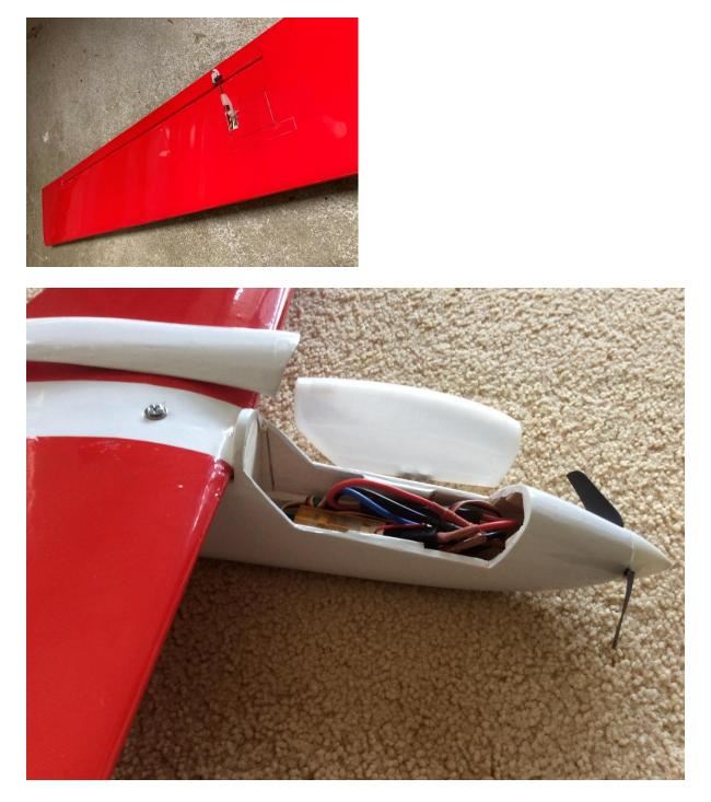
Fit the motor and radio gear. Air holes for motor cooling have not been added at this point in time, but should be considered for motor longevity. If using a 3D-printed canopy, hollow the bottom with a soldering iron to fit the flight battery. Rare earth magnets were used to hold canopy in place. The fairing over the top of the wing is held on with clear tape.
