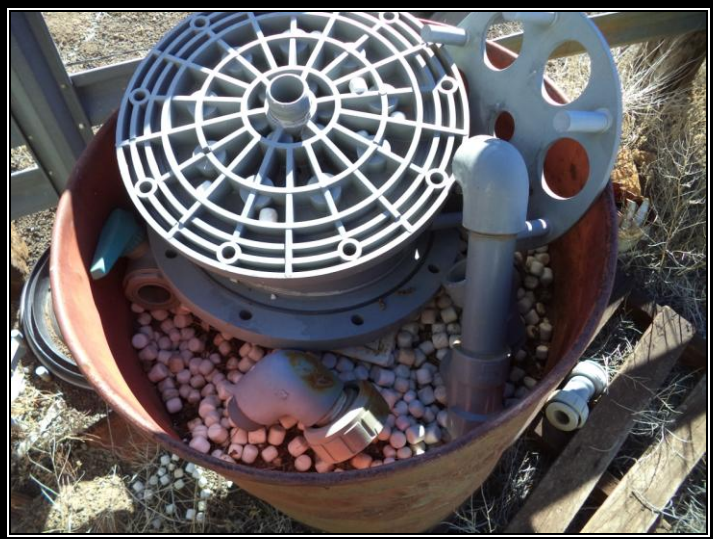
Photo No. 9: View of waste water treatment materials (mostly clay pellets).
