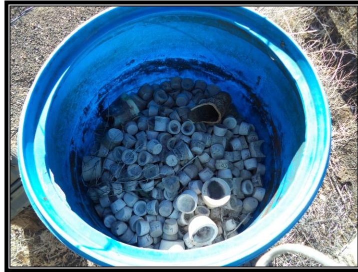
Photo No. 8: Waste assay laboratory materials (cupels and crucibles) in poly drum near southwest corner of Property.
