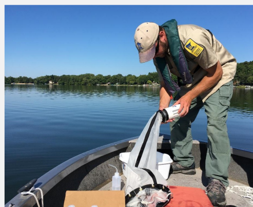
DNR staff collecting samples for veliger testing (microscopic zebra mussels) on Cedar. Lots of nets, bottles, rinsing, and tracking.
