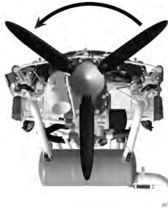
Figure 3: Normal direction of propeller rotation (engine)
