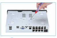
**3** Screw HDD to the bottom
