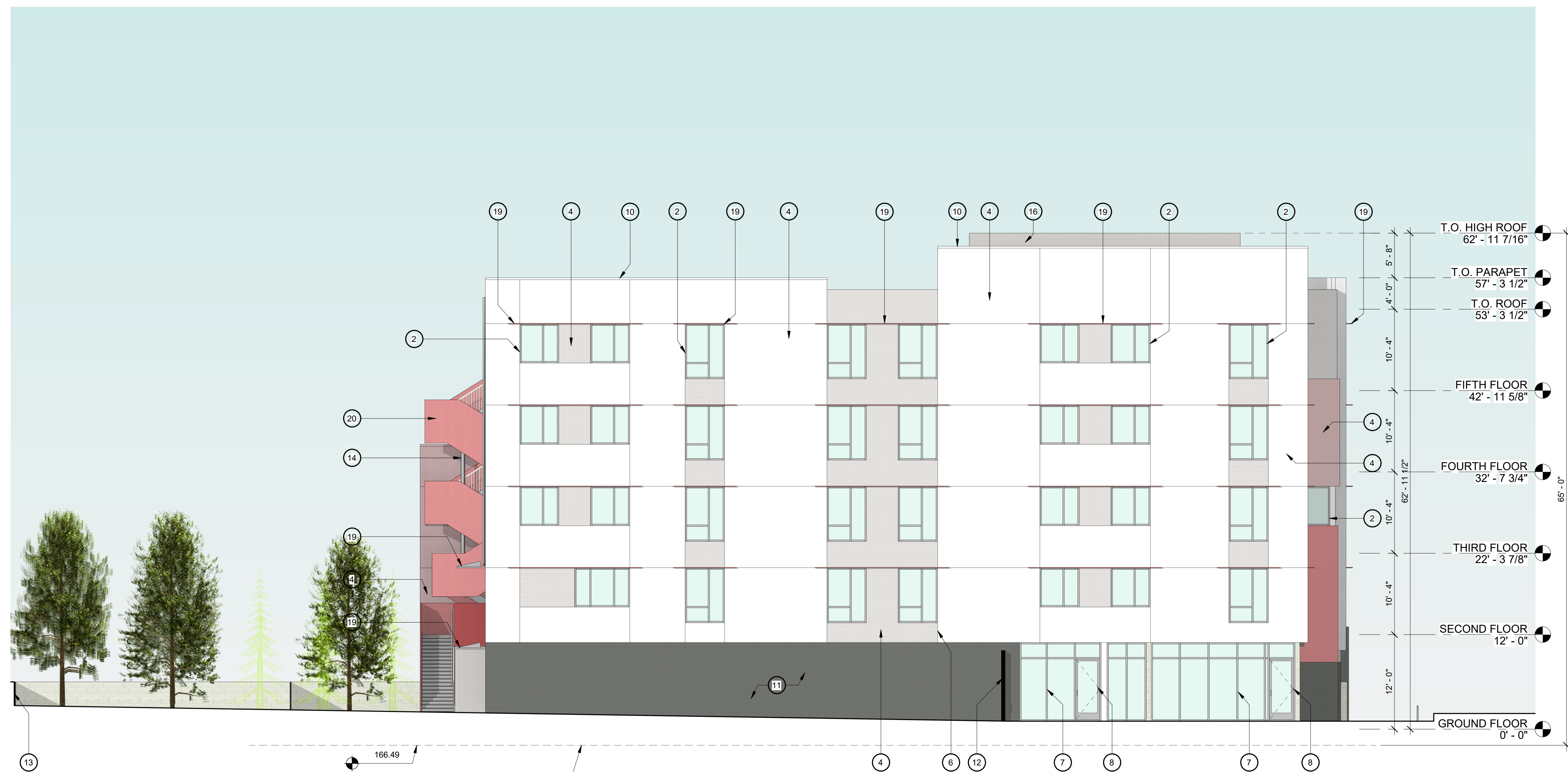
1 SOUTH ELEVATION - SIDE YARD 1/8" = 1'-0"
