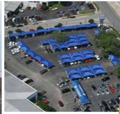
Multiple units grouped together offer maximum coverage using less steel posts offering cost efficiencies for increased shaded areas.
