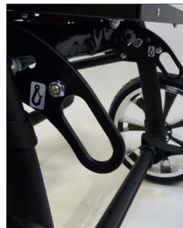
Attachment points, rear according to ISO 7176-19
