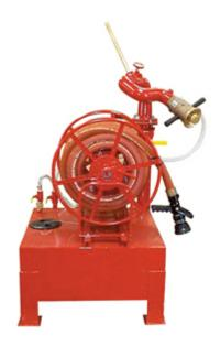
**Minuteman III** packs even more knock-down power than Minuteman II. It features a 3" waterway monitor and a self-educting nozzle capable of flowing at 350 or 500 gpm (1,325 or 1,893 Lpm) with 1% or 3% foam proportioning. Similar to Minuteman II, the monitor and hose line can be used separately or simultaneously with foam or water.
