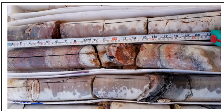
Figure 7. Large calcite breccia with crackle breccia at 351.48m (EA-002).
