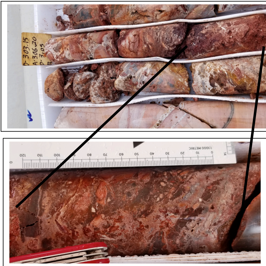
Figure 6. 303m (EA-002) Polymictic breccia to the left with strong silicification, strong limonite and jarosite alteration below carbonaceous limestone unit.
