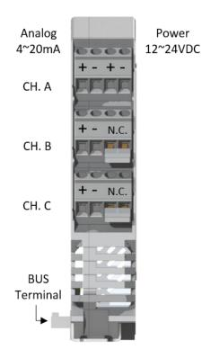
The transmitter is connected into the current loop by output terminals on the device. The pairs of terminals on the left side of the housing are isolated 4-20mA analog outputs. The analog output top pair is for Channel A, the middle pair is for Channel B, and the lower pair is for Channel C.
