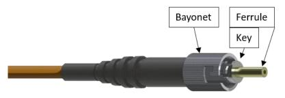
When mating the ST connector to the receptacle on the transmitter, the key must be properly aligned with the slot before insertion. The purpose of the key is to prevent the ferrule from rotating. The bayonet lock is then engaged by pushing and twisting until it reaches the end of its travel. When locked, the bayonet spring prevents the probe from disconnecting.
