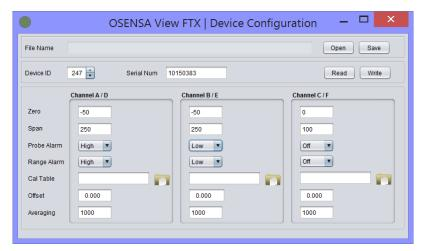
For instance, a Zero value of -50 in Channel A will mean that the analog output will be 4mA when the probe connected to Channel A reads -50°C. If the span is set to 250, then the analog output will read 20mA at 200°C (since -50 + 250 = 200). By setting the Probe Alarm High, the analog output for that channel will read 22.5mA if the probe becomes damaged or disconnected. Similarly, if the Range Alarm
