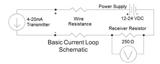
The 4-20mA outputs must be loop powered with a supply voltage between 12 VDC and 24 VDC. The label on the top of the transmitter indicates the polarity. It is important not to reverse the polarity, as this may cause permanent damage to the device.
