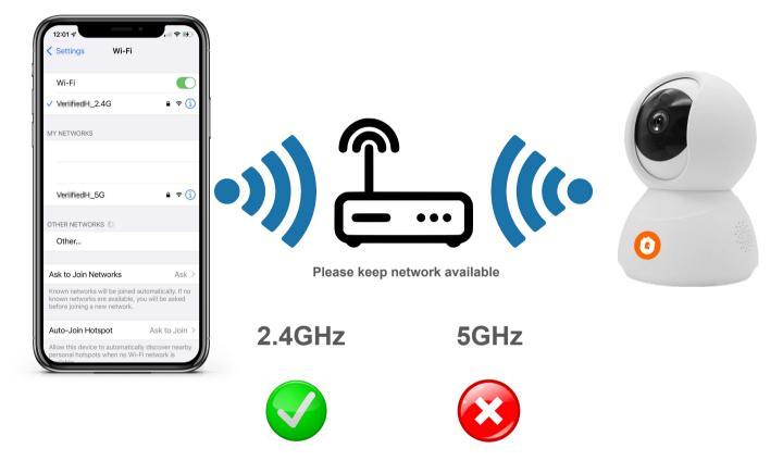
The router supports the 2.4GHz WiFi (doesn't support the 5GHz), and is connected to the WiFi network. Please set the parameters of the router before connecting the WiFi network, and record the SSID and password of your WiFi.
