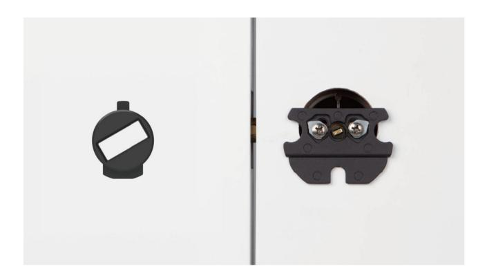
Select the correct adapter based on your deadbolt's tailpiece. If the adapter fits the tailpiece but does not fit in smart lock's motor, flip the adapter and try again. Place the adapter in the motor.
