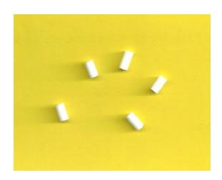
Replacement for the oft missing white pointers for Johnson knobs. These are 0.125-inches in diameter and 0.250-inches long. Normally, these "force fit" into the knob. If necessary, they can be secured with a small drop of "super glue inserted into the knob hole.
