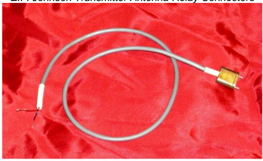
HC6/U style plug for connecting antenna relays to many Johnson transmitters including the Valiant and Ranger series.
