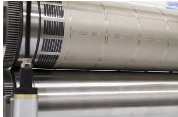
Figure 5: Close-up of the gap between the magnetic and the anvil cylinder
