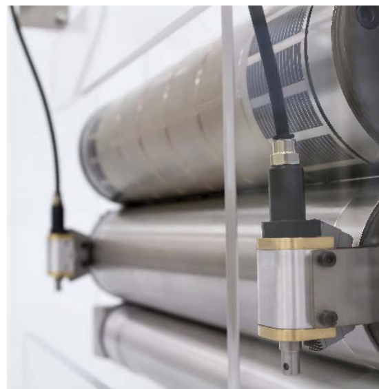
Figure 6: The adjustable anvil cylinder Wink SmartGap permits high-precision gap adjustment
