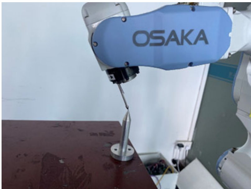
Point 4: The robot returns to zero point with the tool hand end vertical
