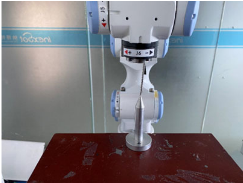
Point 3: The robot rotates 35° around the B-axis on the basis of the first point
