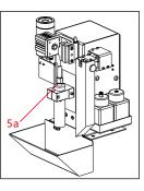
9.1.3 Place the welding torch above the cleaner, make sure the welding torch nozzle at the center of the reamer and parallel to the reamer.
