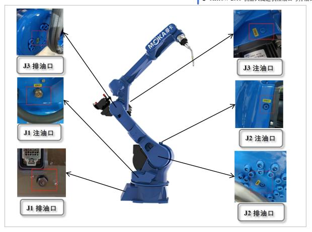
• MR12-2010 Robot reducer oil filling port and oil drain port
