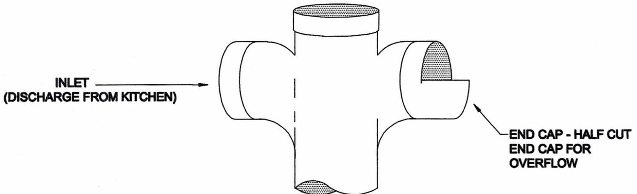
INLET FLOW DISTRIBUTION TEE FOR USE IN ALL GREASE INTERCEPTORS AND OIL/WATER SEPARATORS.
