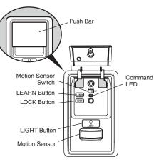
SYNCHRONIZE THE DOOR CONTROL: To synchronize the door control to the garage door opener, press the push bar until the garage door opener activates (it may take up to 3 presses). Test the door control by pressing the push bar; each press of the push bar will activate the garage door opener.
