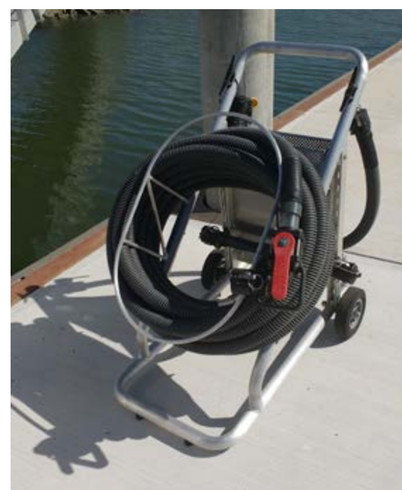
In-slip hose cart at Westpoint Harbor Photo by SFEP
