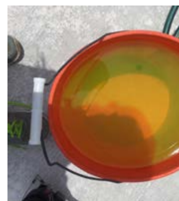
Dye tablet dissolving in 5 gallon bucket of water Photo by TBF
