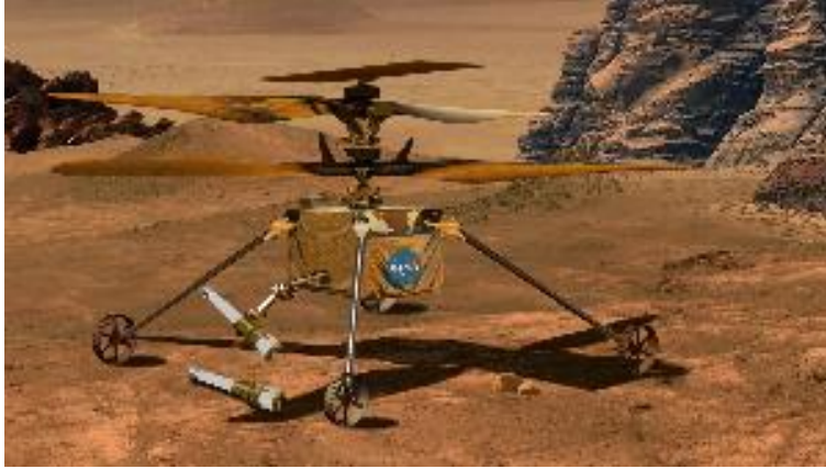
An illustration of one of the Sample Recovery Helicopters slated to fly to Mars as part of the Mars Sample Return Campaign. (Image credit: NASA/JPL-Caltech)
