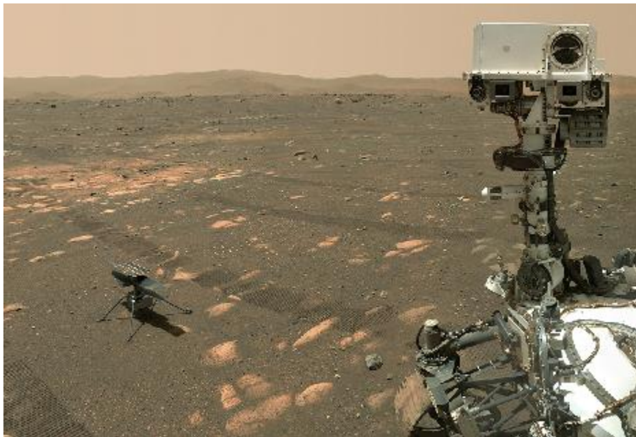
The SuperCam instrument (upper right) on NASA's Perseverance rover includes a microphone, which picked up sounds from the instrument's laser and from the whirling blades on the Ingenuity helicopter (left).
