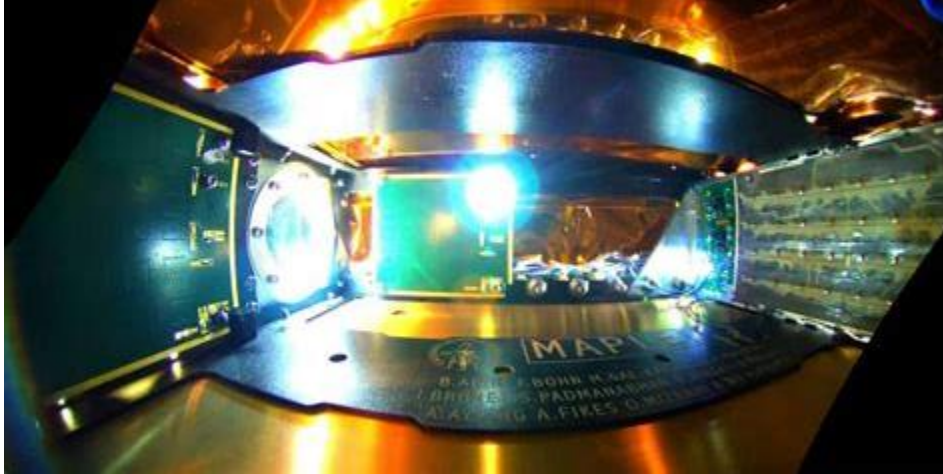
A view from inside MAPLE, which will demonstrate wireless power transmission in space. The top receiver is receiving power in this picture, and it is lit by this wirelessly transmitted power. Caltech
