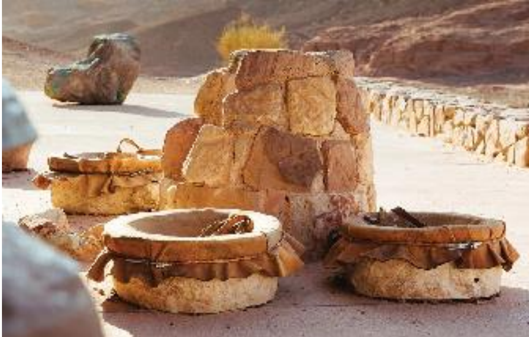
A reconstruction of a smelting furnace with bellows. Ore placed in the charcoal-burning chamber disintegrates. Molten slag drains out; copper remains. Yadid Levy
