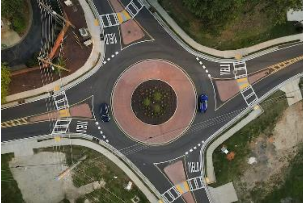
Modern roundabouts can have one or two lanes, and usually have four exit options. AP Photo/Alex Slitz
