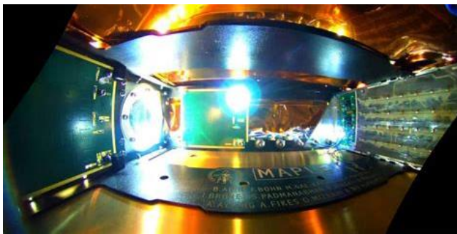
A view from inside MAPLE, which will demonstrate wireless power transmission in space. The top receiver is receiving power in this picture, and it is lit by this wirelessly transmitted power. Caltech
