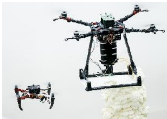
BuilDrones (R) 3D print their material during flight, and ScanDrones (L) continuously measure their output for quality control.
