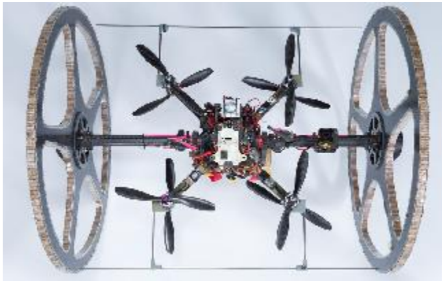
Team CoSTAR's Rollocopter uses a quadrotor system to fly or roll along on two passive wheels. When it meets an obstacle while rolling, it can simply fly over it. Credit: NASA/JPL-Caltech
