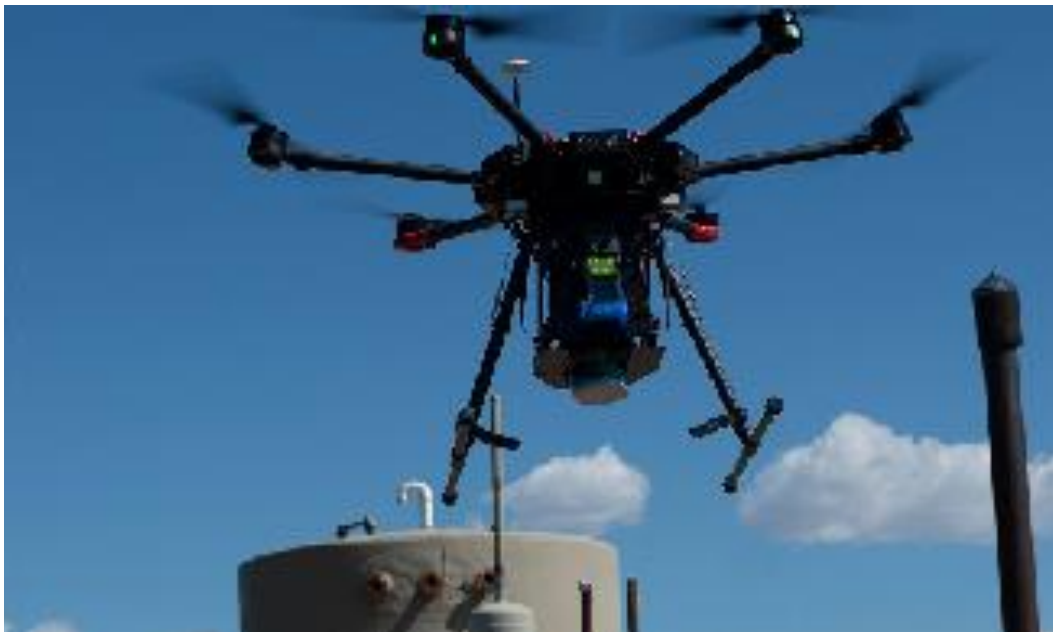
A drone sniffs for methane in Colorado. (Image credit: Sean F. Boggs / Environmental Defense Fund)
