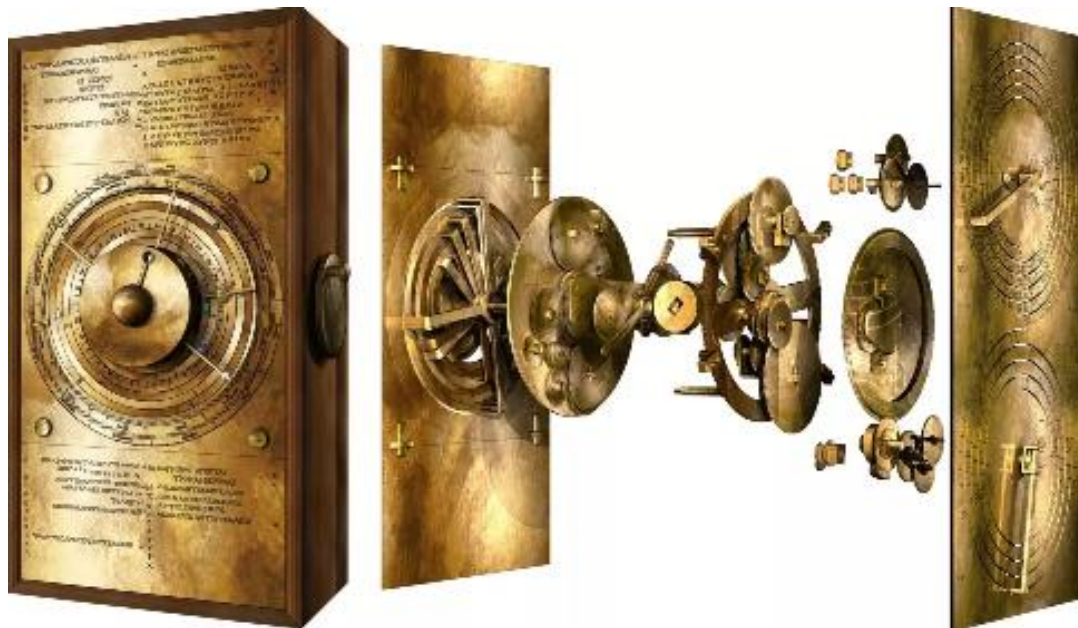
An 'exploded' view of the Antikythera mechanism. (Image credit: Tony Freeth/UCL)
