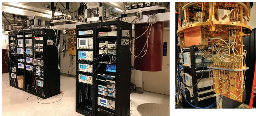
FIGURE 2.6 Laboratory apparatus for a contemporary superconducting qubit system. SOURCE: Courtesy of Dr. William Oliver, Lincoln Laboratory.
