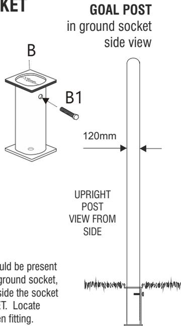
Grey area on diagram denotes the space that should be present once goal is inserted in socket. When fitting any ground socket, tape the top over to prevent concrete dropping inside the socket DURING INSTALLATION OF THE GROUND SOCKET. Locate Upright locking screw to the back of the post when fitting.
