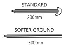
Longer pegs are to be used on sandy or Soft ground earth. **A risk assessment of soil conditions suitability should be carried out when anchors are to be used.**
