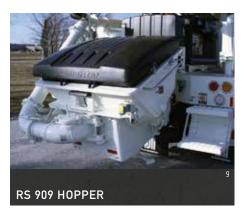
Putzmeister's robust, yet lightweight EZ Clean Out RS 909 hopper is engineered for performance and durability. Offering 19.4 ft³ (550L) capacity, the hopper uses one remixer paddle motor and grate-mounted vibrator. The multi-piece grate features bolted connections that allow for easy maintenance. An innovative RFID safety switch incorporated in the hopper disables the machine when the grate is opened.
