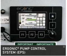
The computer-aided EPS constantly monitors and regulates the operation of the concrete pump and truck engine. The electronic regulation of this system means the pump always runs at peak performance. EPS results in more productivity and greater efficiency with less for the operator to worry about. The color Ergonic Graphic Display (EGD) provides EPS monitoring from one convenient location.
