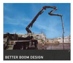
Putzmeister's "smart design" boom incorporates welding seams below the edge of maximum stress. The new 38Z-5 rectangle boom design minimizes boom bounce, and is easier for the hoseman to maneuver. The boom features more straight pipe for a less stressful concrete flow and longer wear on parts. The Z-Fold configuration handles space-restrictive areas and can pump even when the boom is not fully extended.
