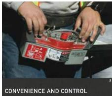
The Automatic Frequency Management (AFM) system on the standard HBC proportional radio remote ensures minimal interference with other frequency transmitters. A fully proportional cable remote is also standard. Unlike other remote control systems, the radio and cable remote systems are independent, offering redundancies to ensure proportional operation with either the radio or cable remote.
