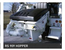
Putzmeister's robust, yet lightweight EZ Clean Out RS 909 hopper is engineered for performance and durability. Offering 19.4 ft<sup>3</sup>. (550L) capacity, the hopper uses one remixer paddle motor and grate-mounted vibrator. The multi-piece grate features bolted connections that allow for easy maintenance. An innovative RFID safety switch incorporated in the hopper disables the machine when the grate is opened.
