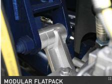
Fully removable, Putzmeister's modular bolt-on flatpack and hydraulic system combine versatility and servicing convenience. This simple design allows for cost-effective, minimally labor intensive pump cell replacement for upgrades, repairs or as part of a maintenance program.
