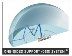
For enhanced job site versatility, Putzmeister's unique OSS system allows the operator to reduce the outrigger extension on one side of the unit to create a smaller overall machine footprint. Utilizing a series of sensors, OSS enables the unit to maintain a defined and safe 180-degree working envelope on spacerestrictive sites that demand a larger boom.
