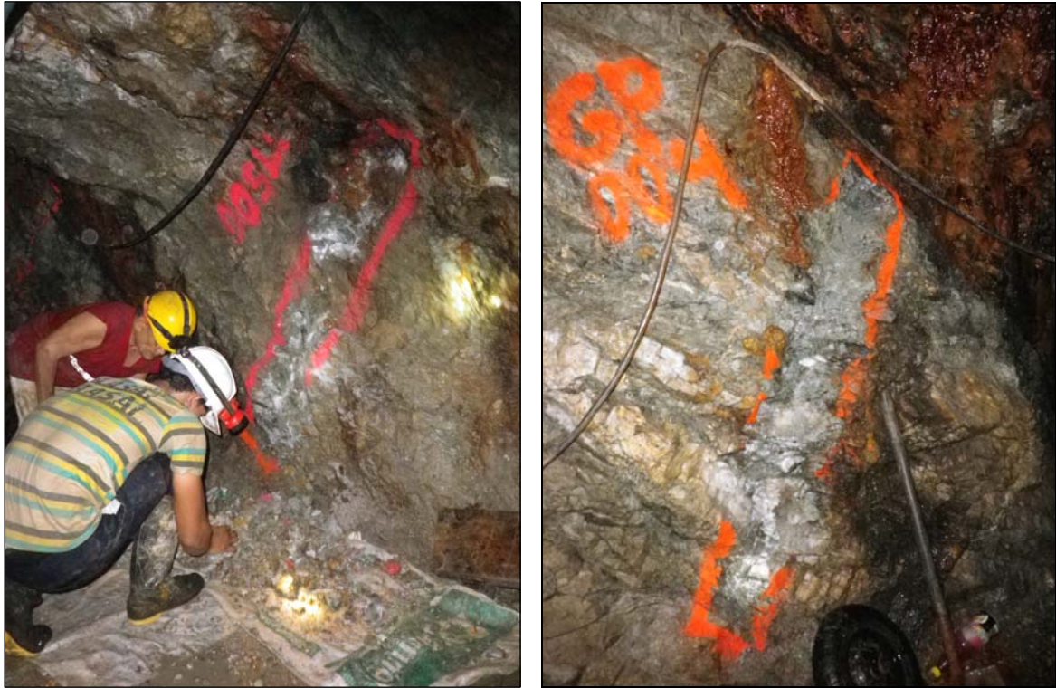
Fig. 11.1.- On the left: Sample gathered on a tarp to avoid pollution (sample GP-005 bis). On the right: Channel on mineralized quartz vein (sample GP-004).
