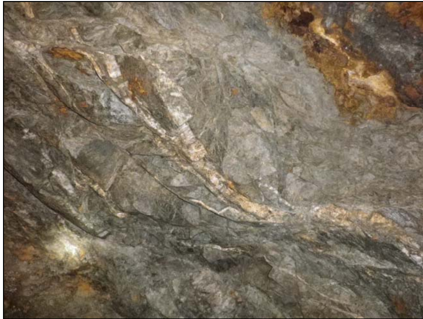
Picture 7.3. Aphanitic mafic rock in the structure between the veins. Central inner area at level 595 (picture 1 m wide).
