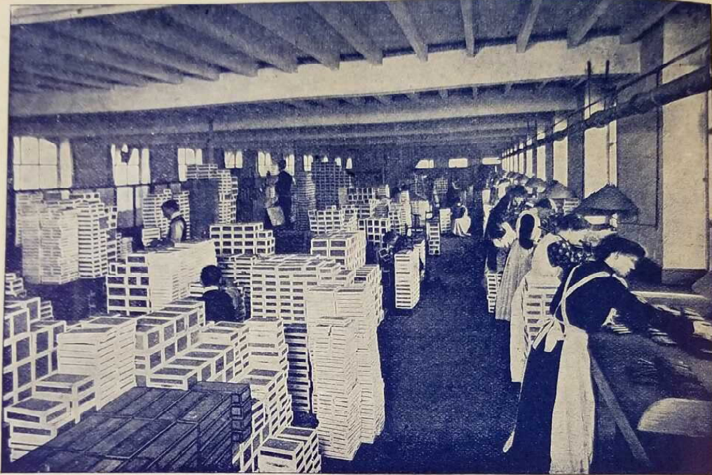
In the Cigar Sorting Department. The Cigars in every brand of "Marsúmas" are carefully graded according to their colour before they are boxed.
