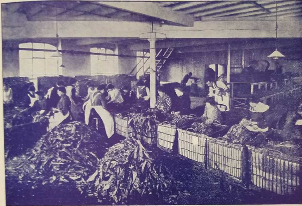
Stripping Virginian tobacco leaf preparatory to cutting the tobacco for "Marsūma" Cigarettes. The stalks and any damaged leaf are removed at this stage and afterwards returned to the Customs, no stalk being mixed with the tobacco.
