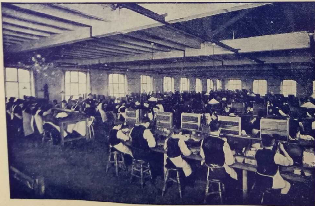
Making "Marsūma" Cigarettes. Every cigarette produced in the Marsūma works is made by hand.
