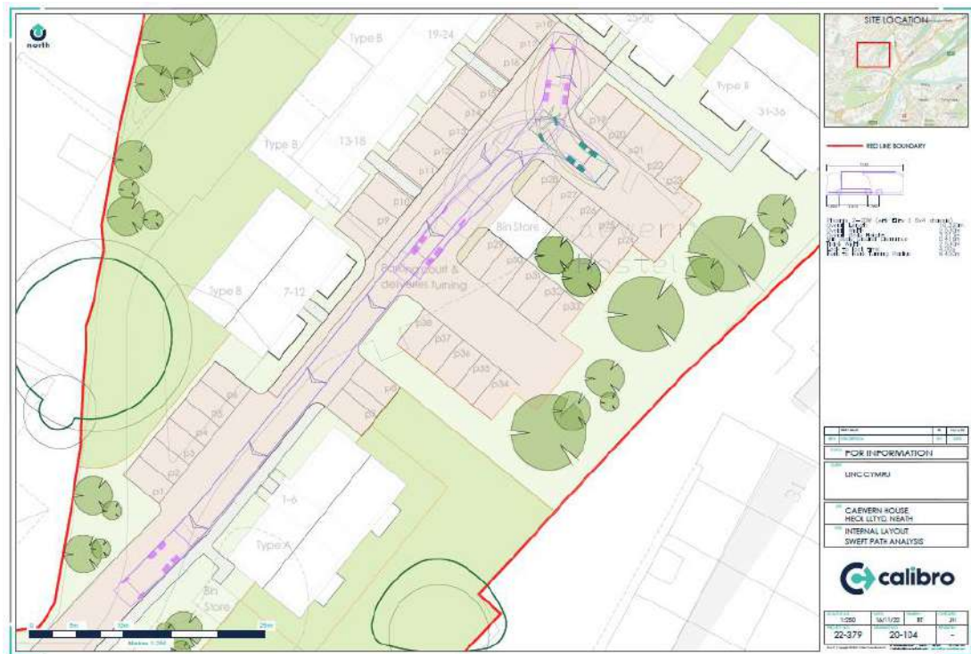
Figure 2.5 Internal Layout Swept-path Analysis
