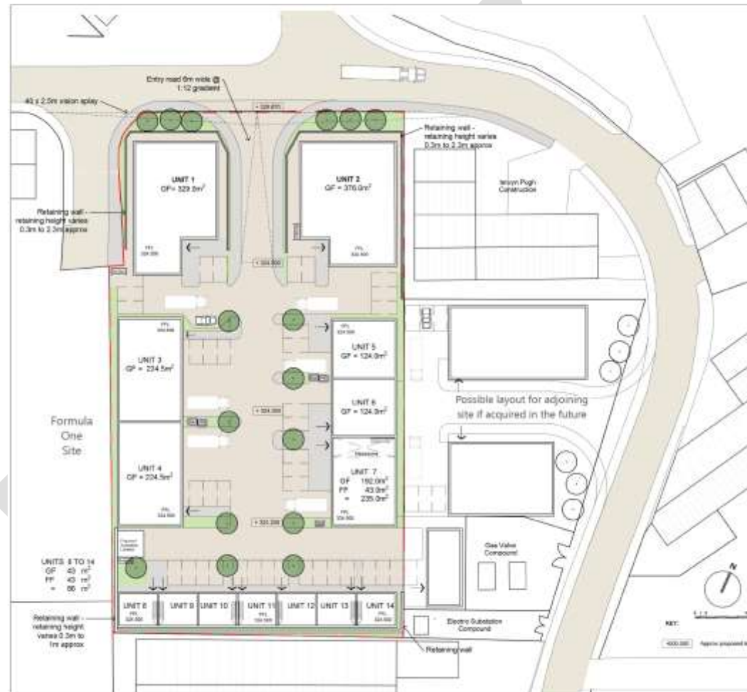
Figure 3: Proposed site layout (please note, works outside of the red line boundary are not covered by this report. Works outside the red line boundary are only potential if the site is re-developed at a later date (please see Feasibility Study, Powell Dobson Architects, 2019 for further information).
