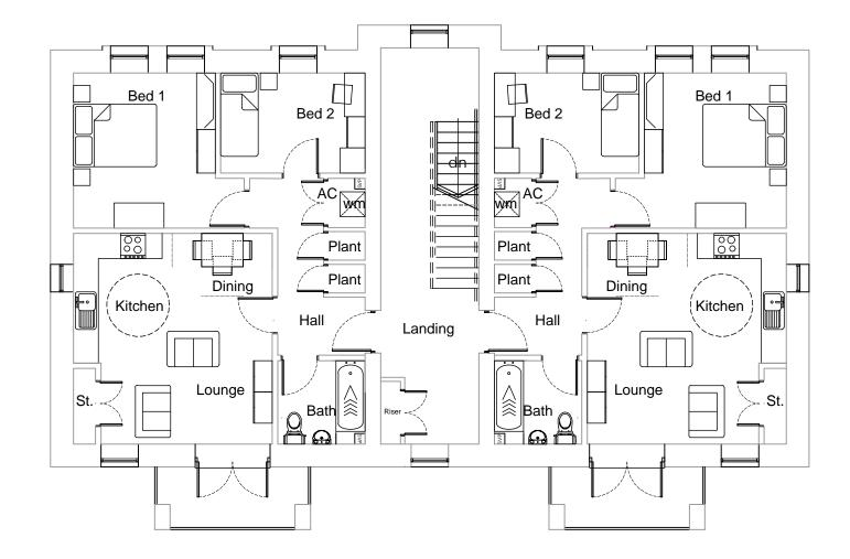
**BUILDING TYPE A: FIRST FLOOR PLAN**
