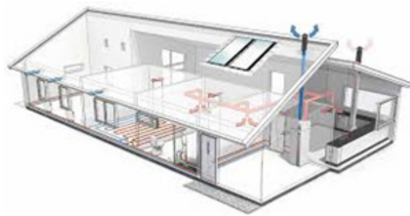
Exhaust Air Heat Pump (NIBE)
