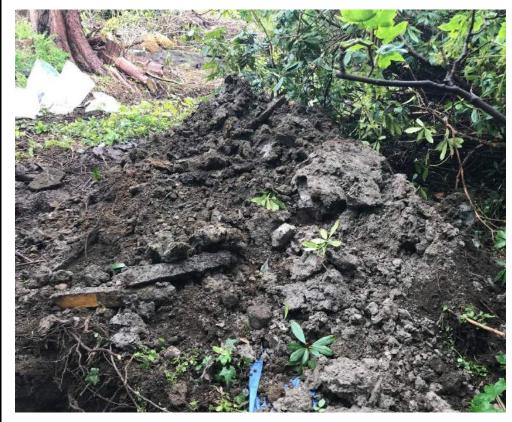
Plate 5: TP202 Spoil after excavation, displaying the Weathered Grovesend Formation bedrock encountered.
