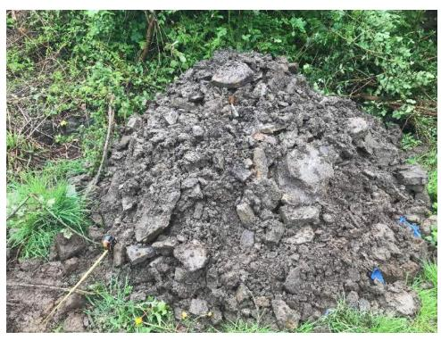
Plate 8: TP203 Spoil after excavation, displaying the Weathered Grovesend Formation bedrock encountered.
