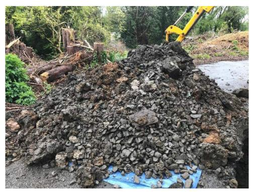
Plate 11: TP205 Spoil after excavation, displaying the gravel fill and Weathered Grovesend Formation bedrock encountered.
