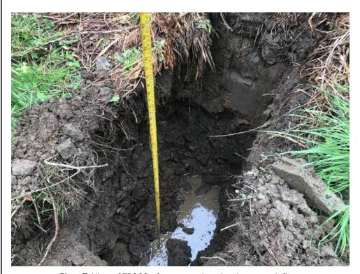
Plate 7: View of TP203 after excavation showing water inflow.
