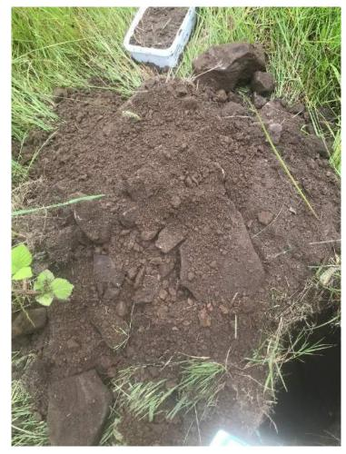
**Plate 15:** HP01 Spoil after excavation, displaying large boulders retrieved from the upper 600mm of material encountered.
