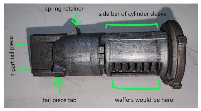
Disassembled cylinder (there is also a key buzzed button, not in pic, that is part of the cylinder)
