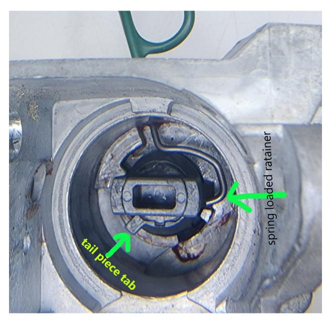
If the spring-loaded retainer is depressed so that it is flush with the outside of the cylinder. The cylinder will release from the housing, but not be able to remove fully from housing because of the tab on the tail piece is not in correct position.
