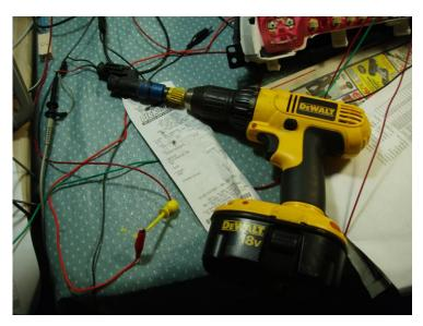
We spun the drill to get it to about 2V P-P on the scope and snapped a shot of the signal:
