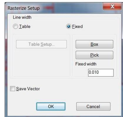
The best way to use this feature is to pick a point on the edge of an existing horizontal or vertical raster line and stretch the box along the line. You can then easily match the width. The length of the rectangle can be any size that is longer than the width as the smallest side is used as the width measurement. A reference rectangle is used instead of a square to make it easier to see. As soon as the second point has been selected, the rasterization takes place.
