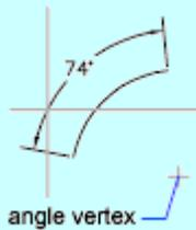
The dimension line is drawn as an arc between the extension lines. The extension lines are drawn from the angle endpoints to the intersection of the dimension line.
