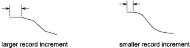
Sketching is captured as a series of independent lines. Setting the SKPOLY system variable to a nonzero value produces a polyline for each contiguous sequence of sketched lines rather than multiple line objects.
