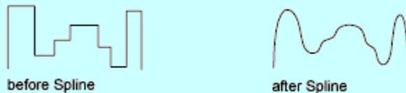
Spline-fit polylines are very different from the curves produced by the Fit option. Fit constructs pairs of arcs that pass through every control point. Both of these curves are different from true B-splines produced with the SPLINE command.
