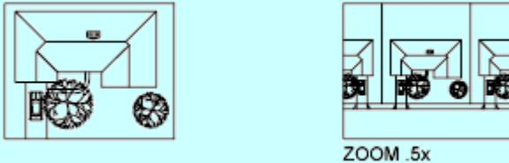
Enter a value followed by **xp** to specify the scale relative to paper space units. For example, entering **.5xp** displays model space at half the scale of paper space units. You can create a layout with each viewport displaying objects at a different scale.
