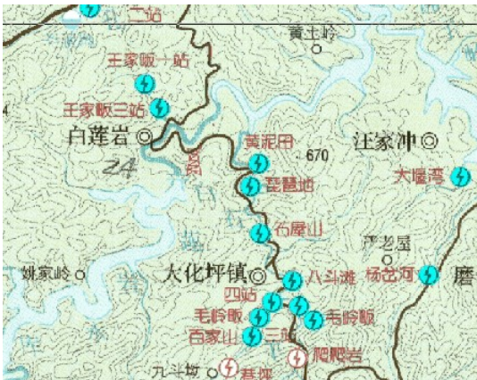
Finding raster objects on an RGB map and placing a semitransparent vector circle on them.
