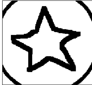
Drawing when RDRAW is ON. Vector circle is drawn and immediately rasterized (note clipping by image boundary)
