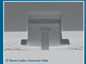
Well-defined 3D resist profile for a T-gate nanostructure with 950k PMMA (bottom) / AR-P 617 / CSAR 62
