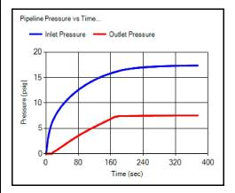
**Graphic Results** - GASPurge displays its results in a graphic chart to visualize the pipeline purging process conveniently. Users can view Flow Rate versus Time, Pressure versus Time, Pipeline Velocity versus Time, and Exit Velocity versus Time.
