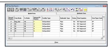
pressures, flow rates, velocities and volumes, and simultaneous reporting of linear and pressure drop per User specified length. Selection sets may be created from within the data reports, allowing unique reporting of User-specified data groups. Hierarchical queries will enable the creation of sub-sets from a previously created selection set.
